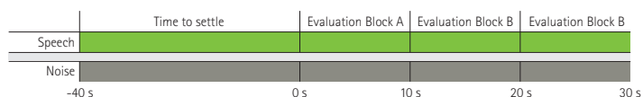
Figure 5. Stimulus presentation: Before each measurements, 40 seconds of the ISTS speech signal (S) and respective background noise (N) were played to allow the hearing instruments to settle. The evaluation period was 10 seconds for each evaluation Block, see methods.
