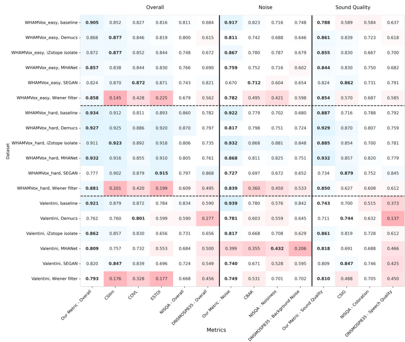
Figure 5. Pearson correlation of various metrics with human ratings on various datasets. Red shades indicate low correlations and blue shades high correlations. The numbers in bold are the highest correlations in each category. For more details refer to Diehl et al. 2022.
